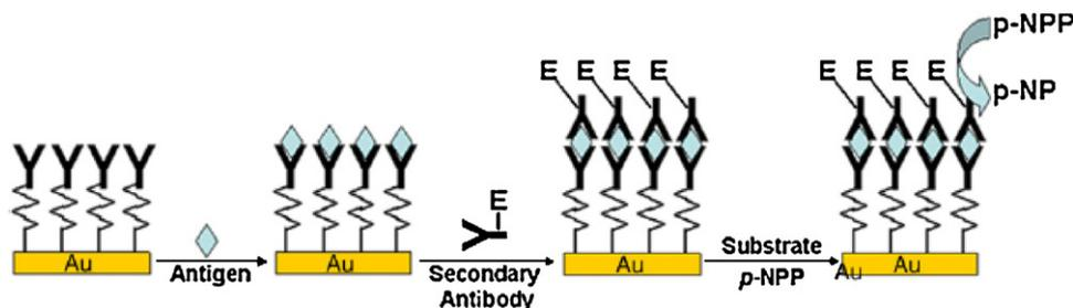
**Fig. 2.** Thiolated antibodies can be used to realize a reproducible and ordered self-assembled monolayer on a gold electrode surface. With this scheme, the thiolated antibody is the recognition element and allow to develop a sandwich assay with the target analyte (here Staphylococcal enterotoxin B) and AP-conjugated secondary antibodies. Reproduced with permission from [23]. Copyright (2007) from Elsevier B.V.
