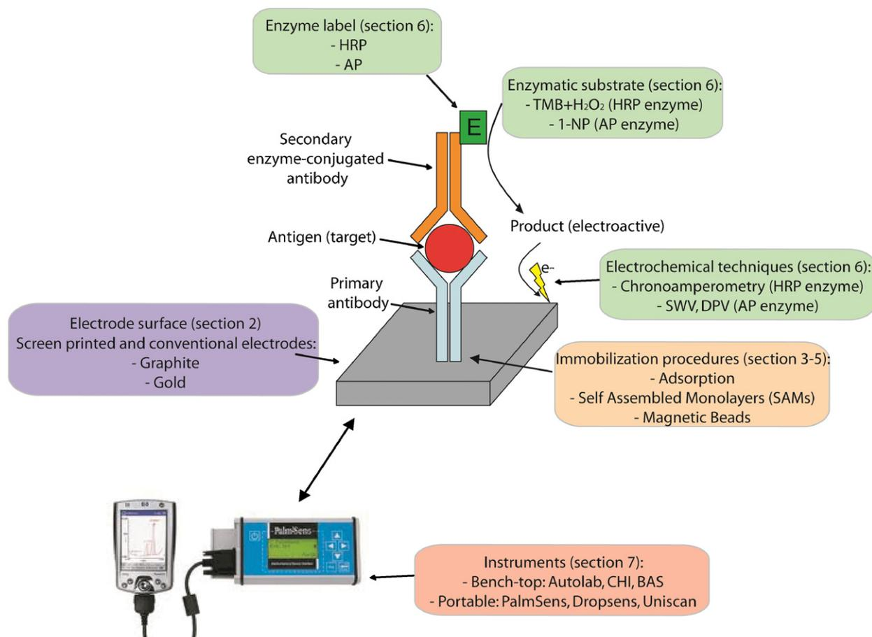
**Fig. 1.** General overview of the main components of an electrochemical immunosensor. In this scheme, for the sake of clarity, we have depicted a generic immunosensor based on a sandwich format. The components that should be considered in the development of an electrochemical immunosensor are briefly overviewed. In this review we highlight the reasons to choose among the multiple options that are available to the public in terms of electrodes, instruments, enzymatic labels and reagents.
