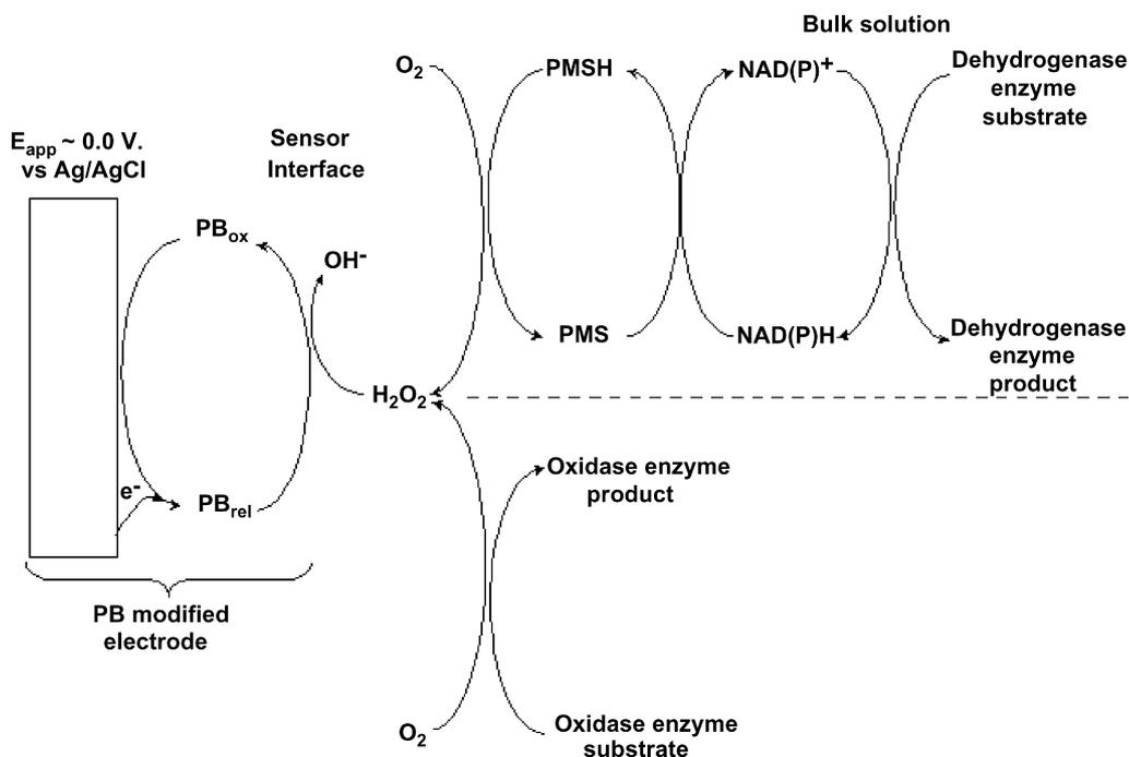
Scheme 1. Schematic representation of the system adopted for NADH detection. In the upper part of the scheme is shown the reaction chain for the detection of NAD(P)H as in the case of a NAD(P) dependent dehydrogenase enzyme. In the lower part of the scheme is shown the classic reaction utilised in the case of an oxidase enzyme. In both cases, the final product is  $\text{H}_2\text{O}_2$ , which is measured at the Prussian Blue modified electrode at an applied potential of ca. 0.0 V vs. Ag/AgCl.
