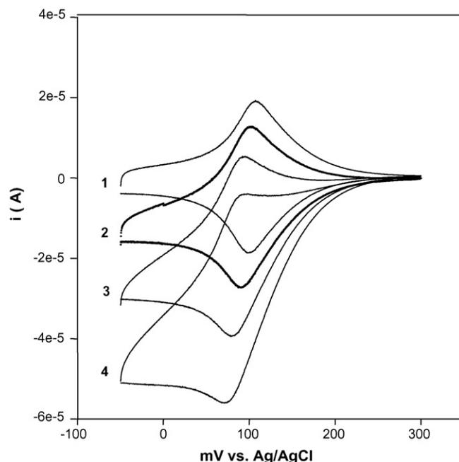
Fig. 1. Cyclic voltammetry of Prussian Blue modified electrode. Phosphate buffer  $0.05 \text{ mol L}^{-1}$  + KCl  $0.1 \text{ mol L}^{-1}$ , pH 7.4. Scan rate  $50 \text{ mV/s}$ . CV obtained in buffer + PMS  $10^{-4} \text{ mol L}^{-1}$  in absence (1) and presence of  $2.5 \times 10^{-4} \text{ mol L}^{-1}$  (2),  $5 \times 10^{-4} \text{ mol L}^{-1}$  (3) and  $10^{-3} \text{ mol L}^{-1}$  (4) of NADH.
